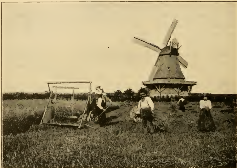
HARVESTING IN 1831. McCormick's first successful horse-reaper — the first improvement upon the cradle scythe. The "self-binder" was a later feature. From a photograph based upon a "reconstruction" by the International Harvester Company.
